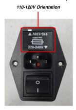
The fuse cartridge holder on some Fusion units may differ to what's described above. Always check the fuse information on the rear of your physical unit to verify you are inserting the correct fuses when changing the operational voltage.
