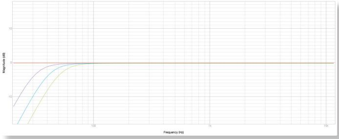
HPF Plots - OFF, 30Hz, 40Hz, 50Hz.
