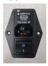
Fusion has a linear power supply. The AC mains fuse is located on the rear panel next to the AC mains connector. The orientation of the mains fuse cartridge the 2 fuses used within the cartridge will dictate the operational voltage; this can be either 220-240V or 110-120V AC power.
