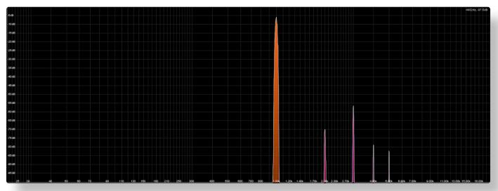
Example of additional harmonics generated using a 1kHz tone. ('High' Density)
