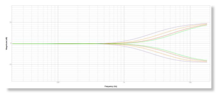
Maximum Gain plots of Violet EQ - 8 kHz, 12 kHz, 16 kHz and 20 kHz.
