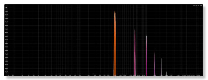
Example of additional harmonics generated using a 1kHz tone. ('Low' Density)
