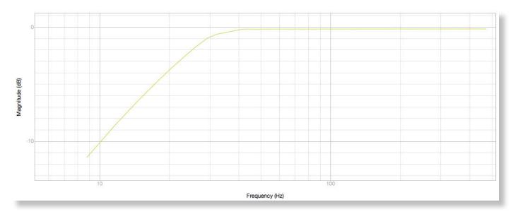
Typical Low Frequency Rolloff of Transformer with +16dBu on input.
