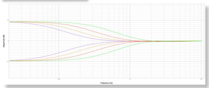
Maximum Gain plots of Violet EQ - 30 Hz, 50 Hz, 70 Hz and 90 Hz.
