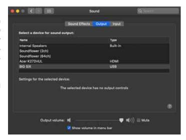
To manage the routing of the Mac System Audio to BiG SiX, this is set-up using the AUDIO DEVICES menu of the AUDIO MIDI SETUP menu, typically found in the Applications/Utilities Menu of OSx e.g.
