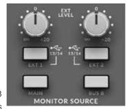
to be sourced from USB Returns 13/14 and 15/16 respectively. These switches over-ride the External Input TRS Jacks.
