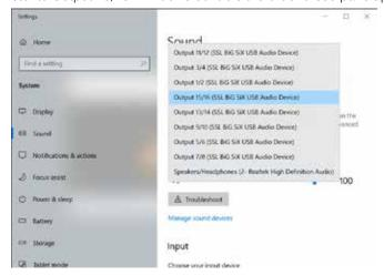
The inputs to the PC from BiG SiX are similarly labelled Input 1/2, etc. up to Input 11/12, the remaining Inputs are labelled according to their source, i.e. Input Bus B L/R and Input Main Mix L/R these are USB inputs 13/14 and 15/16 respectively.
