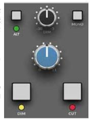
The MONO switch sums the monitor output to Mono with a -3 dB level drop.
