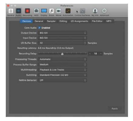
The outputs from BiG SiX now appear as discrete sources for the input routing of the DAW again an example for Logic Pro is shown on the right...
