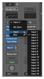
Similarly the inputs to BiG SiX appear as discrete sources for the output routing of the DAW again an example for Logic Pro is shown on the right...
