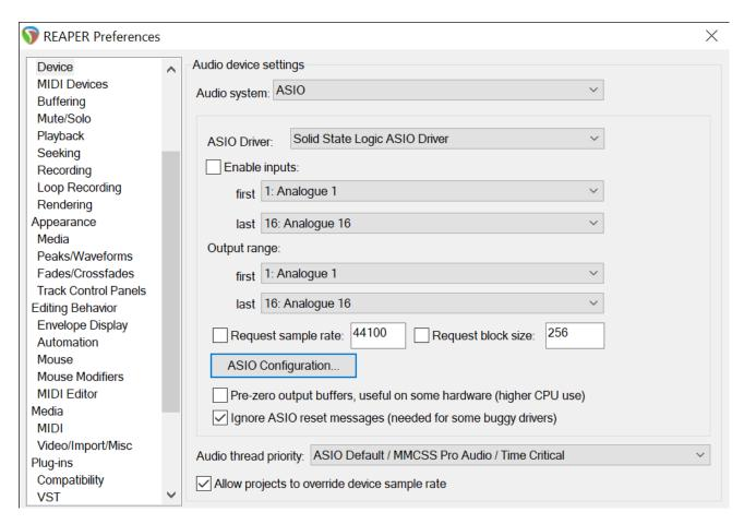
For the best and most flexible performance with DAW's ASIO is the preferred choice. For other Windows audio formats, the driver arranges the USB signals to and from BiG SiX in pairs, the output from the PC to BiG SiX are labelled as Output 1/2, Output 3/4, etc. to Output 15/16. Windows controls the order these pairs appear, so they may not be in sequence!
