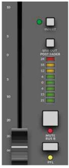
Following the EQ and compressor in the channel signal flow is a fully balanced insert point. In common with larger SSL consoles, the Insert Send is always active, while the Insert Return switches into the signal path when selected.
