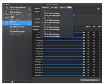
Also in this menu is where the Mac's audio routing to the BiG SiX may be set-up, using the CONFIGURE SPEAKERS menu on this page. For example, you may want to configure the Mac output to send to EXT 2 on BiG SiX, in which case routing the 'Speakers' to Outputs 15/16 will enable this, shown in this diagram on the right...
