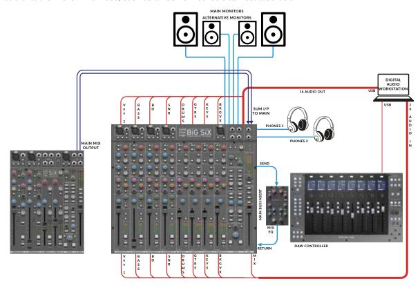
Main Mix Bus Block Diagram showing 'Sum I/P to Main' connection on left hand side.
