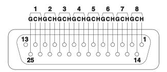
DB-25 Line Level Audio Connectors for Channels 1-8, 9-16, 17-24, 25-32 (4 sets of seven female connectors)
