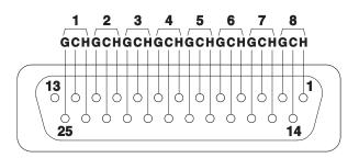
DB-25 Line Level Audio Connectors for Channels 1-8, 9-16, 17-24, 25-32 (4 sets of seven female connectors)
