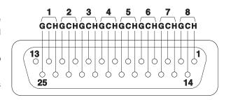
DB-25 Line Level Audio Connector Layout for the Master Section (all female connectors)
