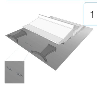
Ensure that the legs, leg fixings and console are conveniently located for assembly. In the diagram on the left the foam base tray is in position behind the console to provide a cushioned base to protect the rear of the console and the floor when fitting the legs.
