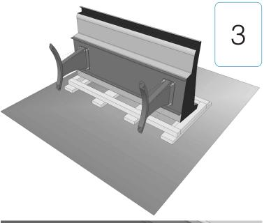
With the console carefully resting on it's rear, use the eight M8 nuts supplied to attach the legs onto the studs protruding from the console base.
