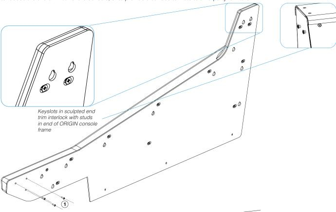
Removing the end trim starts with removing the three cross headed screws that secure the front buffer/armrest (1 in the diagram above) and the three 2mm hex headed retaining screws (2 in the diagram on the right) on the bottom edge of the trim. With these six screws removed the trim can be gently slid up vertically to align the keyhole slots with the locating lugs and then removing the trim horizontally.
