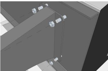
With the legs attached securely, the console can be lifted to it's final position.
