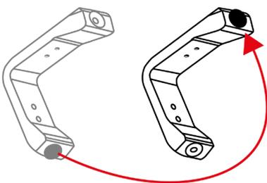
2. Rotate the stands so that the short side fixes to the chassis
