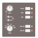
Locate the console oscillator (above the TFT screen), press **OSC ON** and select the **PINK ON** button; the default level for the console's pink noise output is +4dBu RMS. This calibrated level can be adjusted using the 'Pink' trim pot below the **Level** control.
