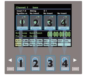
Holding down the **OPTION** button while editing a plug-in parameter will show a 9-character version of the parameter value at the top of the Plug-In Editor display.:
