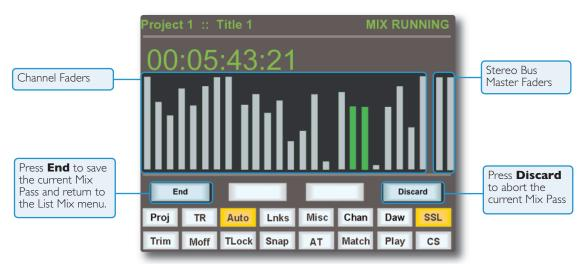
The system saves a Global Static reference mix of the fader levels and cut status at their positions when the **Execute** key is pressed. This is useful because it allows you to locate before the start of the mix and recover your original levels (i.e.reference mix). Also, if you are writing automation in a section that had no previous mix data, when you drop out of write the faders go back to their original levels.
