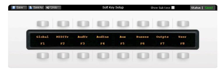
Above you can see the assignments for User 2. (The assignments on User 2 control display options for the Matrix faders.)
