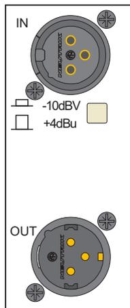
The module input and output gains can be set to operate at a nominal level of either +4dBu or -10dBV, using a switch on the connector panel. To select the appropriate level for the equipment you are connecting to, please check the operating manual for your mixer or DAW. The switch should be released for +4dBu operation: push it in for -10dBV operation.
