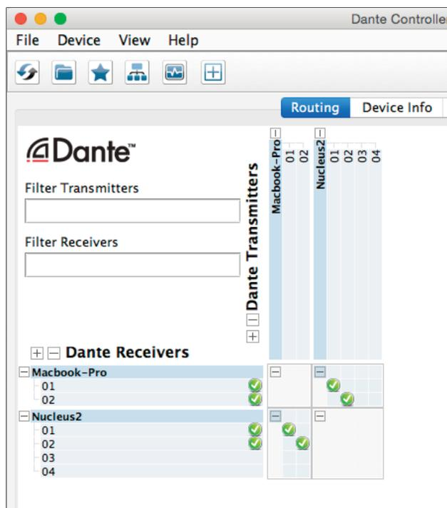
*The SPDIF I/O on channels 3&4 is only available on the Dante Network at low sample rates (44.1/48kHz). At higher sample rates (88.2/96kHz) only the analogue I/O on channels 1&2 will be available.*
