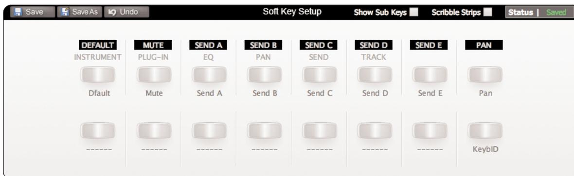
Mode switches 1-8 on the left-hand side come pre-assigned to the functions printed beneath them on Nucleus<sup>2</sup>:
