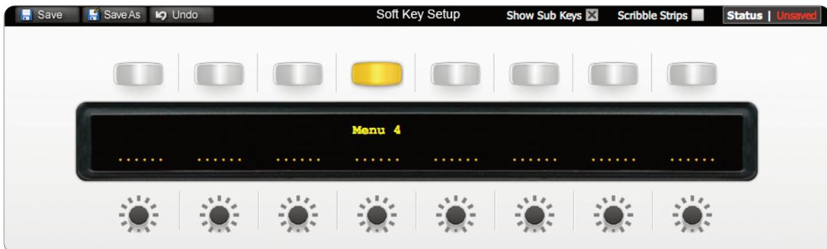
You can now assign functions to the V-Sel switch in the same way as you would for any other soft key, as described previously. Once you have created the soft key assignments for this menu, selecting another top row button that has been assigned as a menu selector will switch the on-screen scribble strip and V-Sel switches to that menu selector. Once you have completed the soft key assignments within all the menus, deselect the **Show Sub Keys** box to return the window to normal operation.
