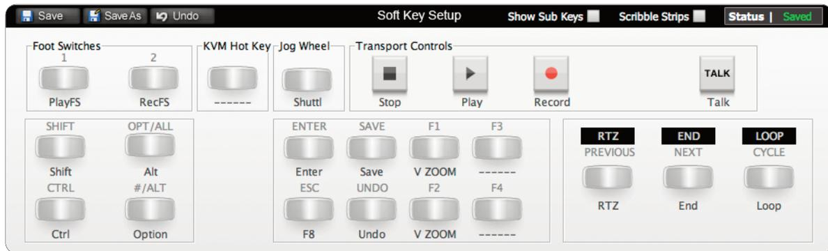
All of these switches (with the exception of F3 and F4) come pre-assigned to the functions printed on the Nucleus<sup>2</sup> control surface.
