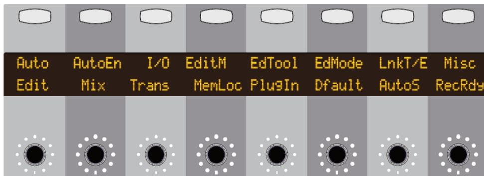
The two soft key sets are called **User 1** and **User 2**, and are activated by pressing the **USER 1** or **USER 2** switch, below the Nucleus<sup>2</sup> logo in the centre section. The top row of the scribble strip display indicates the Mode switch function, the bottom row the V-Sel function. To return the Mode and V-Sel switches to their normal functions, deselect both **USER 1** or **USER 2** switches.
