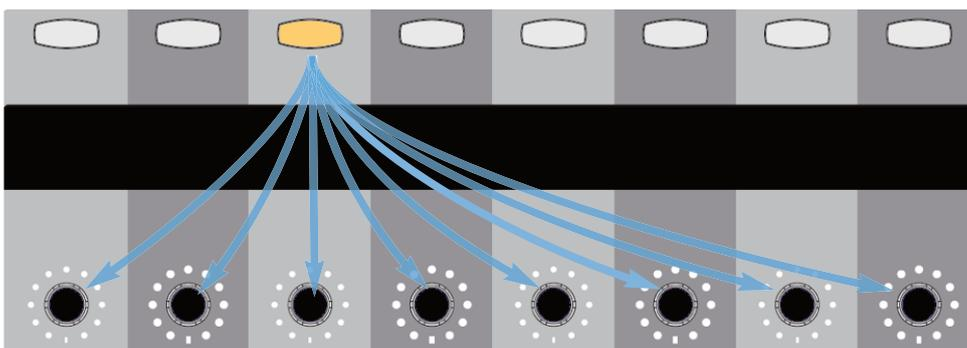
Taking the V-Sel assignments which will be active with no Mode switches selected in to account, the two **USER** soft key sets can be configured to provide access to up to 144 functions. This is of course in addition to all of the other user-assignable switches across the control surface.
