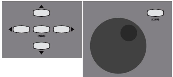
The jog wheel's default function is **'Wheel'**, which is a basic scrolling function in most DAWs. The other modes are **FF/RW** and **+/-** (HUI only timeline scrolling – resolution is controlled by the Timeline format and Nudge value respectively), and **TRACKS** which assigns the channel scrolling function to the jog wheel.
