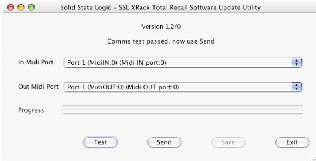
If the test fails check that the correct MIDI port has been selected and that the X-Rack is in software download mode, then repeat the test.
