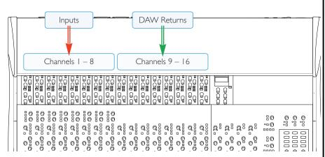
Plug 8 microphones into MIC INPUT 1-8 of XL-Desk. (Using the DB25 to 8 XLR female interface lead, where necessary.)
