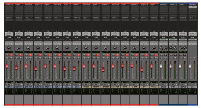
10) Route the sub-groups out of the DAW into the stereo channels of XL-Desk. Route the click track into the final stereo input on XL-Desk and press the **MONO** button. Route these channels to Mix Bus A using the **A** routing button above the **CUT** button.
