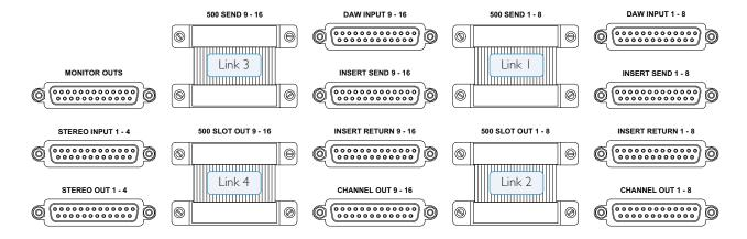
Adding these connectors will link the insert points associated with the 500 button, to and from the 500-series rack.
